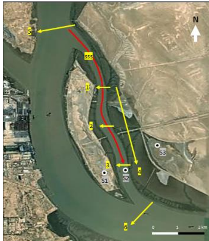
Fig. 2. The SBP (yellow) and SSS (red) track lines as well as the sampler sites
