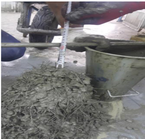
Figure 2: Polyolefin fiber in concrete mix – SikaFiber® Force-6.
