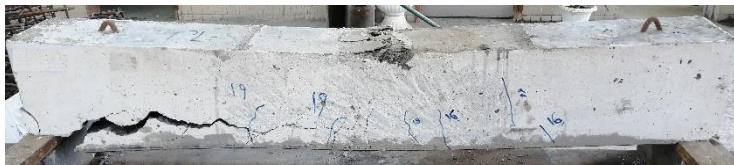
Fig. 15. RB1.0 Beam failure.
