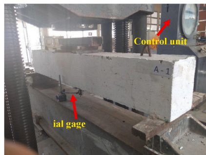
Fig. 6. Details of the test setup.
