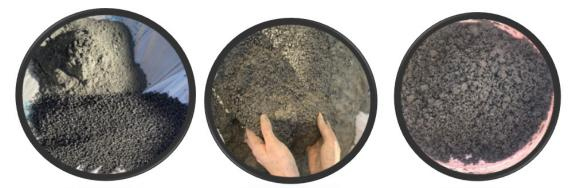
Figure 2. Prepare and mix polyethylene or polypropylene waste pellets with Portland cement
