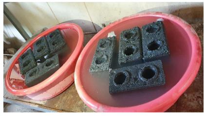
Figure 4. Plastic blocks in water dipping
