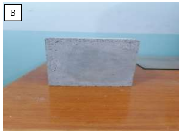
FIGURE 2: (A)The foam process of foam concrete and (B) foam concrete with filler
