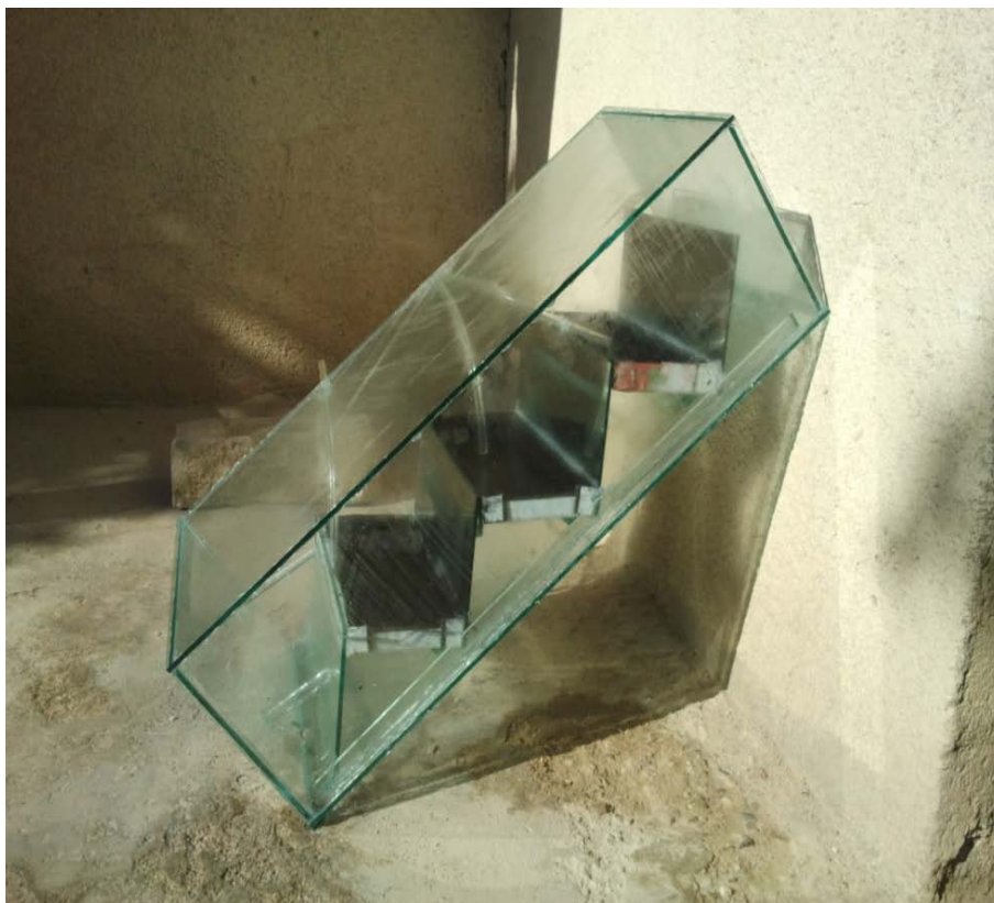
Figure 4: A photographic picture of the Stepped Solar Still (SSS)
