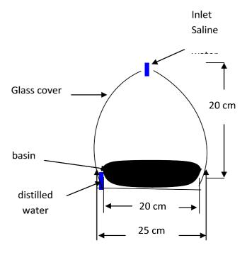
FIGURE 2: A schematic diagram of the Conical Solar Still (CSS).
