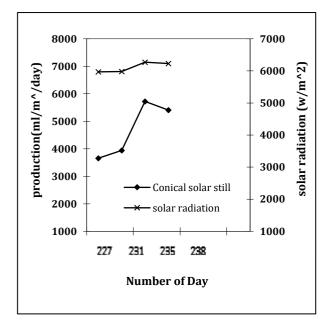
**FIGURE 5:** Daily productivity for the conical solar still with the solar radiation through some days of (August 2023).
