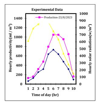
**FIGURE 4:** Hourly productivity of the conical solar still with solar radiation during the day of (15 Aug. and 23 Aug.) 2023.
