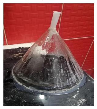
FIGURE 1: A photographic picture of the Conical Solar Still (CSS).
