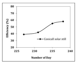
**FIGURE 6:** Thermal efficiency of the conical solar still through some days of (August 2013).
