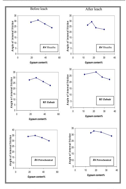
Fig. (7): Relationship between gypsum content and angle of internal friction.
