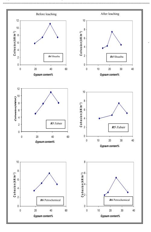
Fig. (5), Relationship between gypsum content and cohesion
