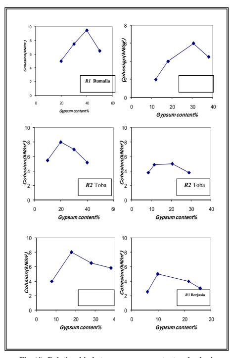
Fig. (4), Relationship between gypsum content and cohesion.
