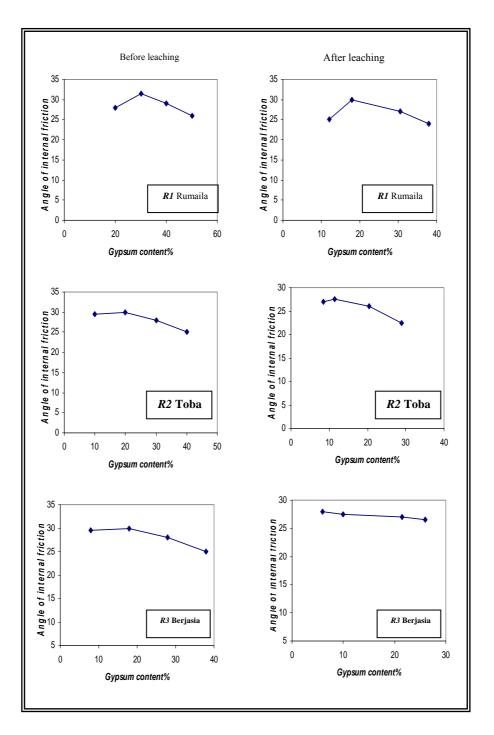
Fig. (6): Relationship between gypsum content and angle of internal friction
