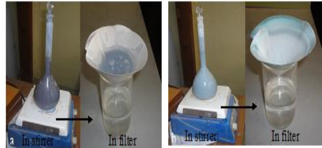
Fig. 2 The photographs of the (a) ZrO 2 -Cu coating powder succeeded on stirrer plate and filter, (b) ZrO 2 -Cu coating powder failure on stirrer plate and filter.
