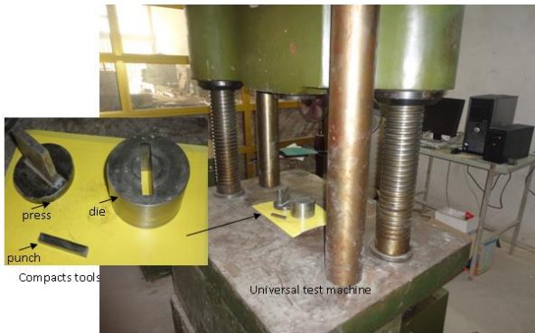
Fig. 5 Computer controlling versatile electronic testing machine and the compaction tools.
