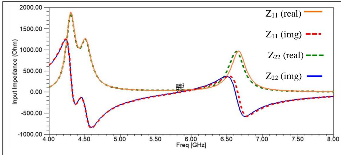
**FIGURE 6.** Simulation results of the input impedances ( $Z_{11}$  and  $Z_{22}$ ) for designed antenna (C5).
