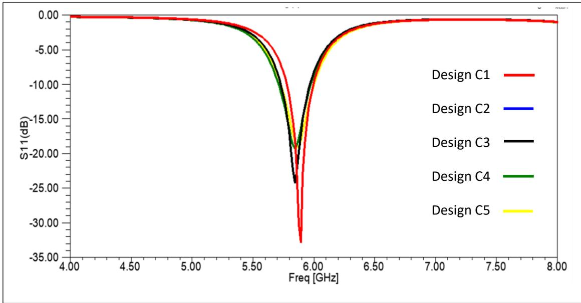
**FIGURE 3.** Simulation results of return loss ( $S_{11}$ ) for the designed antennas in Fig. 1
