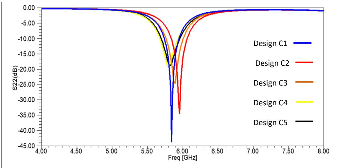
**FIGURE 4.** Simulation results of return loss ( $S_{22}$ ) for the designed antennas in Fig. 1
