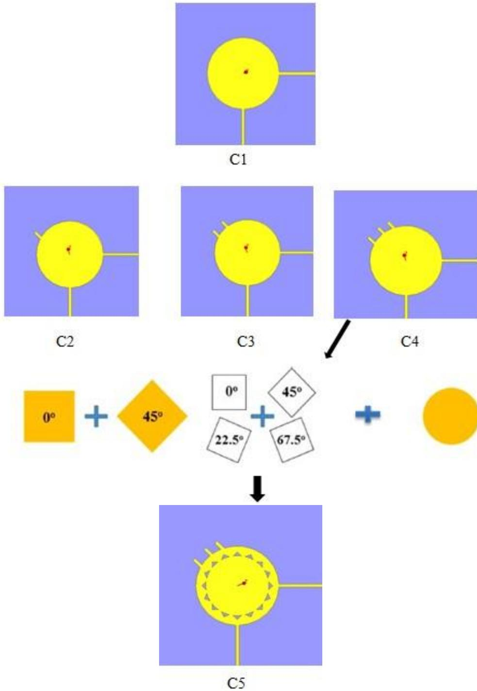
FIGURE 1. Steps designed of the suggested antenna
