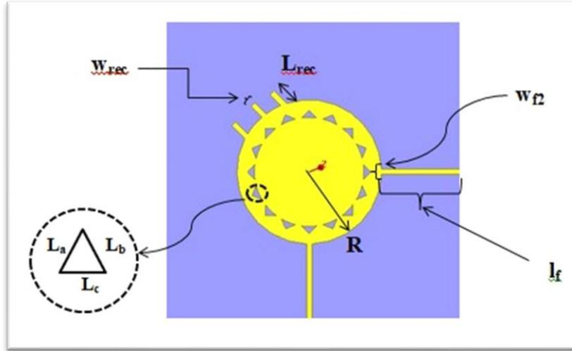
**FIGURE 2.** The geometrical of antenna design C5.
