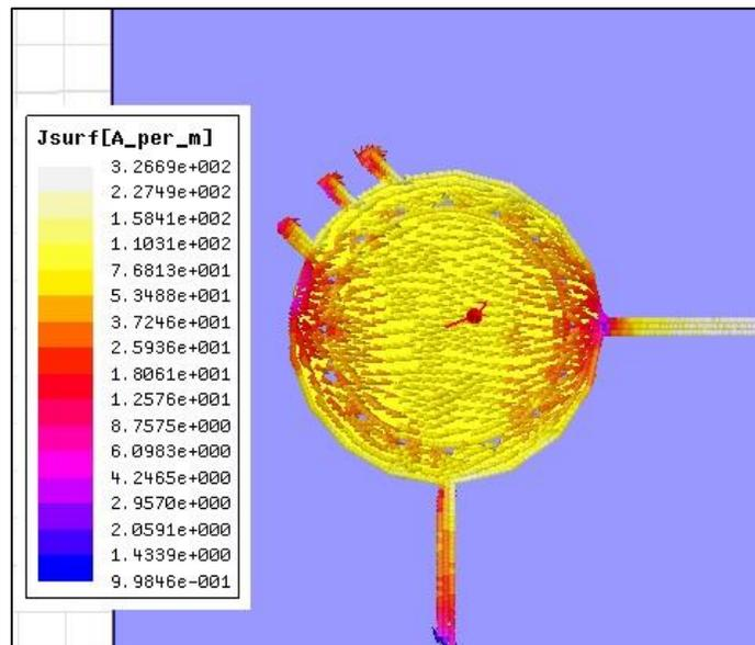
**FIGURE 7.** Electric current distribution simulation on the new suggested antenna (design C5).
