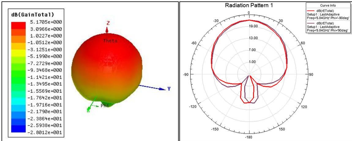
**FIGURE 5.** Simulation results of radiation pattern in the two dimension and gain in three dimension for proposed antenna in Fig.(2), (H-plane black curve and E-plane red curve).
