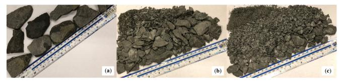
Figure 3. The effect of slaking on mudrock (a) before slaking, (b) after first cycle, (c) after second cycle.
