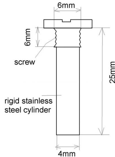
**FIGURE 2** Schematic diagram of electrode
