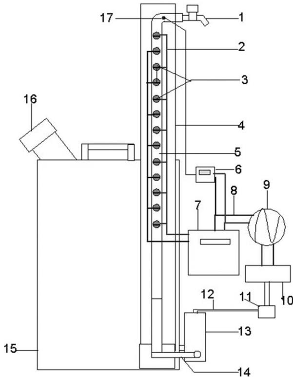
**FIGURE 1** Schematic diagram of CNTJP using AC EF consisting of: 1, tap; 2, electric wire; 3, electrodes; 4, plastic tube cover; 5, pasteurization tube; 6, digital temperature gauge; 7, Variac; 8, electric cable; 9, 220 VAC power source; 10, 220 VAC to 12 VDC power converter; 11, electrical connector; 12, electric cable; 13, DC centrifugal pump; 14, pipe; 15, plastic reservoir; 16, reservoir cap; and 17, thermocouple
