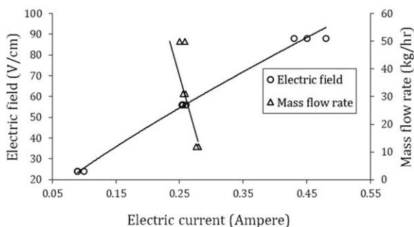
**FIGURE 7** The relationship among the electric field, mass flow rate, and alternating electric current
