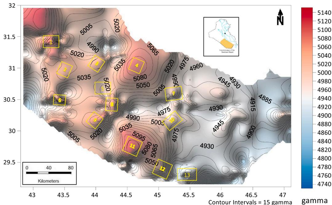
Fig. 13. RTP magnetic map illustrating the possible thirteen sites inside the study area from the total magnetic intensity map of the same area indicates the locations of suitable landfill sites.
