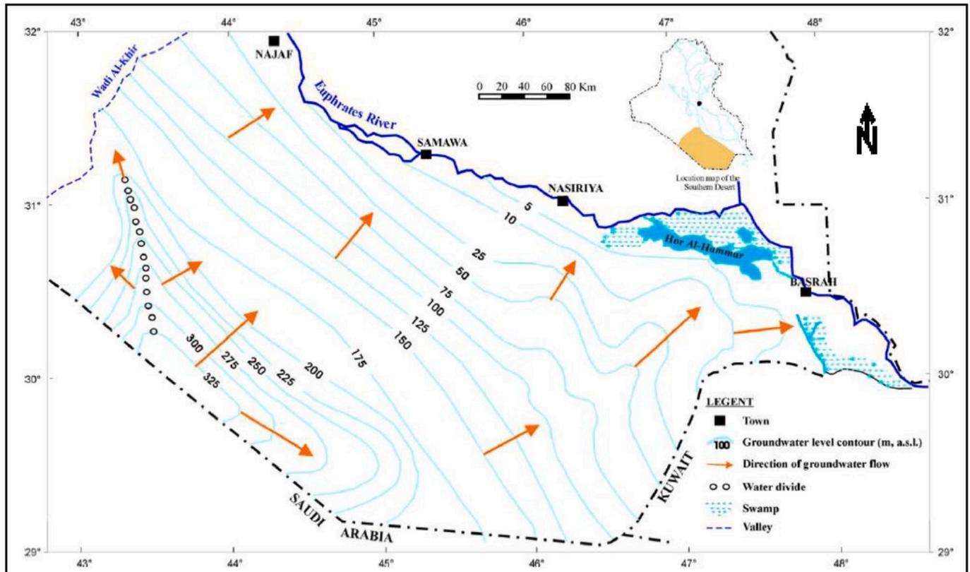
Fig. 4. Hydrogeological map of the Iraqi Southern Desert showing static water level and direction of groundwater flow.
