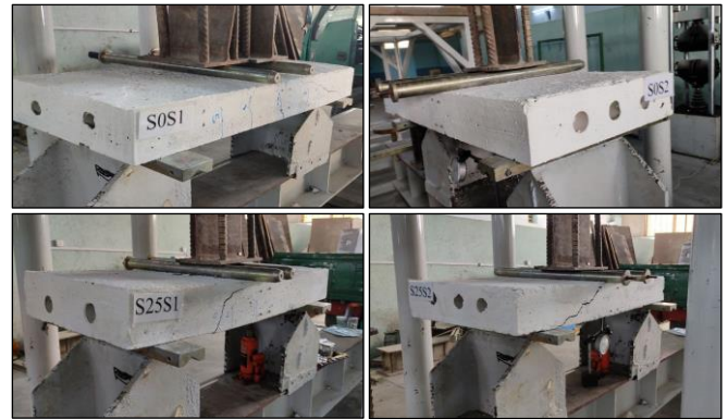
Fig. 4 Crack pattern and failure mode of analyzed RC slabs.
