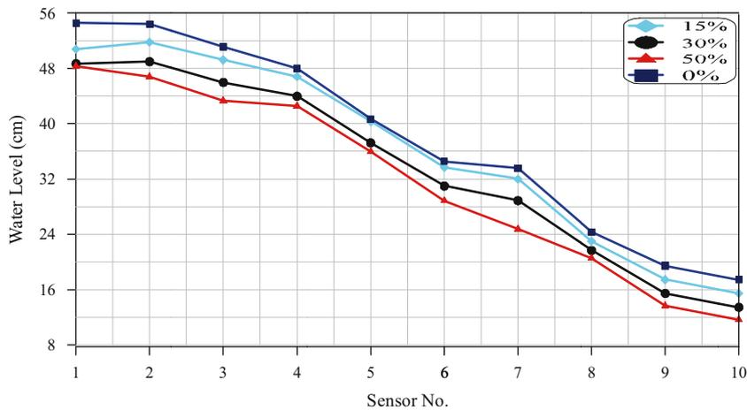
**Figure 13:** Phreatic line of the physical model at steady state condition.
