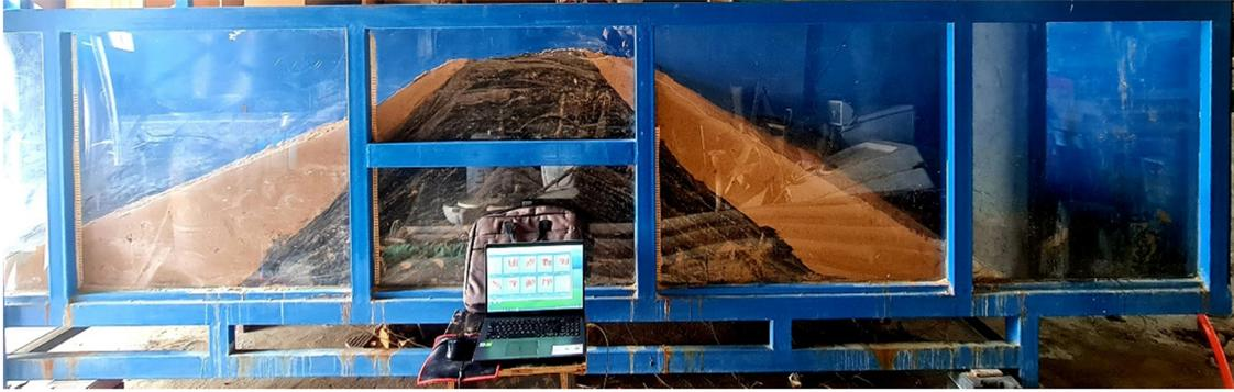
Figure 9: Enhanced homogenous dam model with TRP core at slope 1:1.
