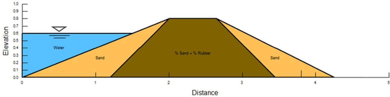
**Figure 4:** Zoned dam type with rubber powder (TRP) core at slope 1:1.
