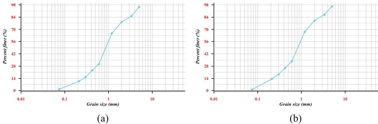
Figure 10: Particle size distribution for dam soil: (a) without TRP and (b) with TRP.
