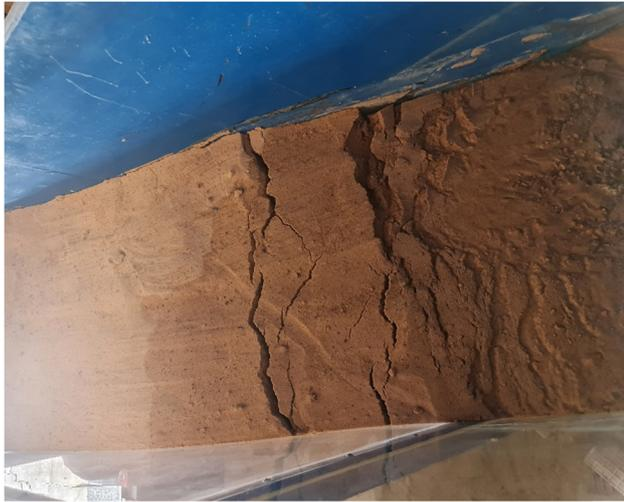
**Figure 12:** Failure in the *D/S* slope of the first model due to seepage line.
