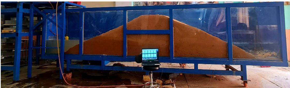
Figure 8: Physical homogenous dam model without TRP core.
