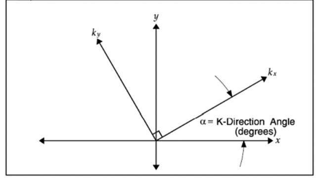
Figure 2: Hydraulic conductivity matrix parameters definition.
