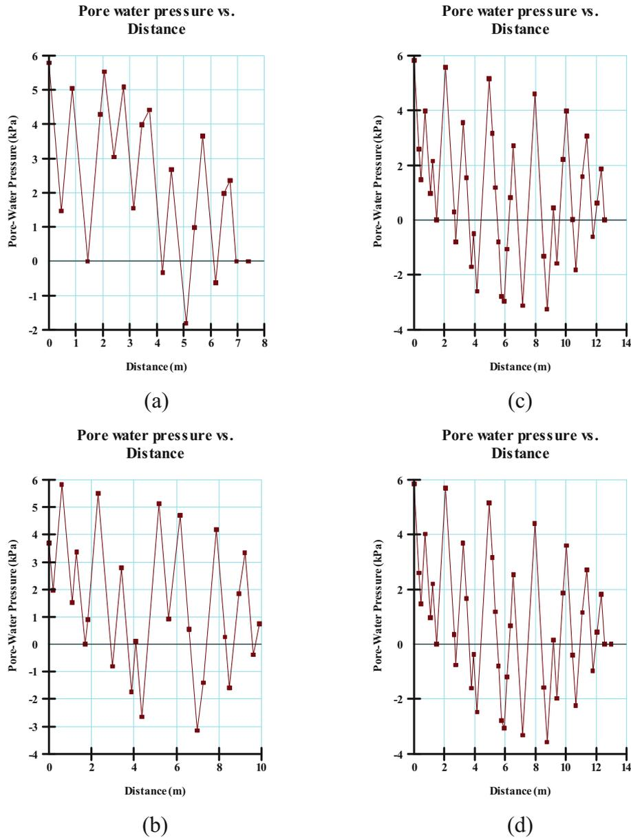
Figure 15: Relation between pore water pressure and distance for four models. (a) without TRP core, (b) with 15%, (c) with 30%, and (d) with 50%.
