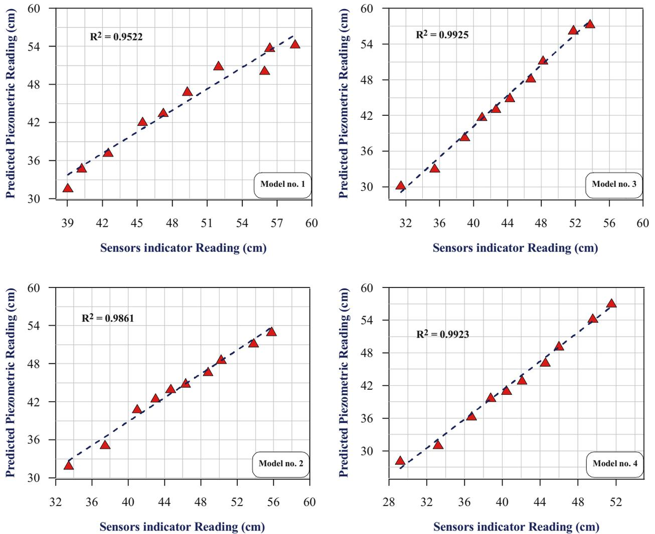
**Figure 16:** Sensors indicator reading and piezometric reading between physical models and SEEP/W.
