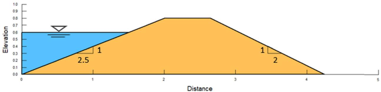
Figure 3: Homogenous dam type without rubber powder (TRP).
