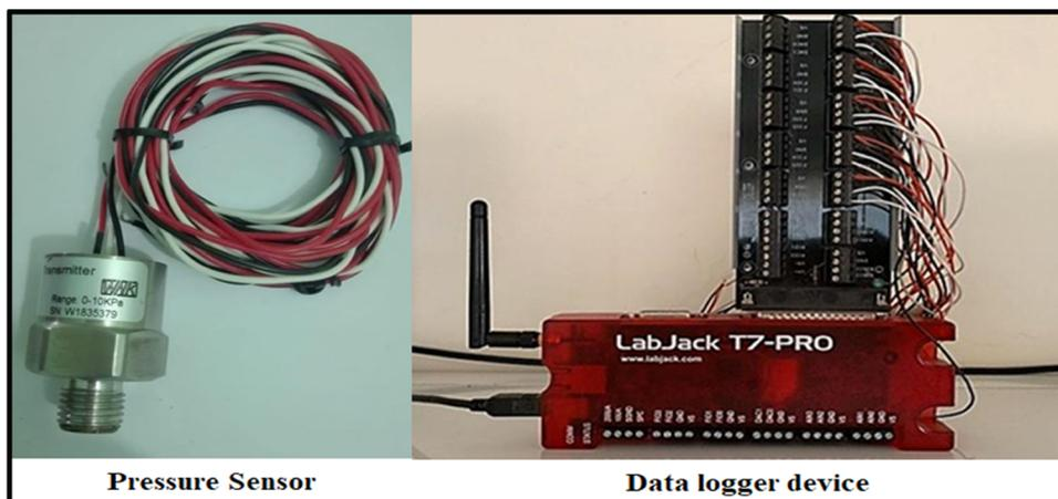
**Figure 5:** The pressure sensor and data logger device.
