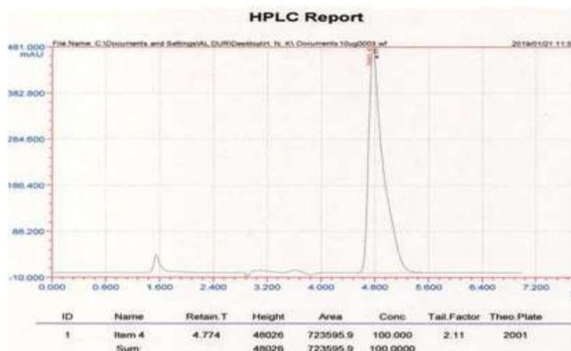
Figure 3: Base Degradation Chromatogram
