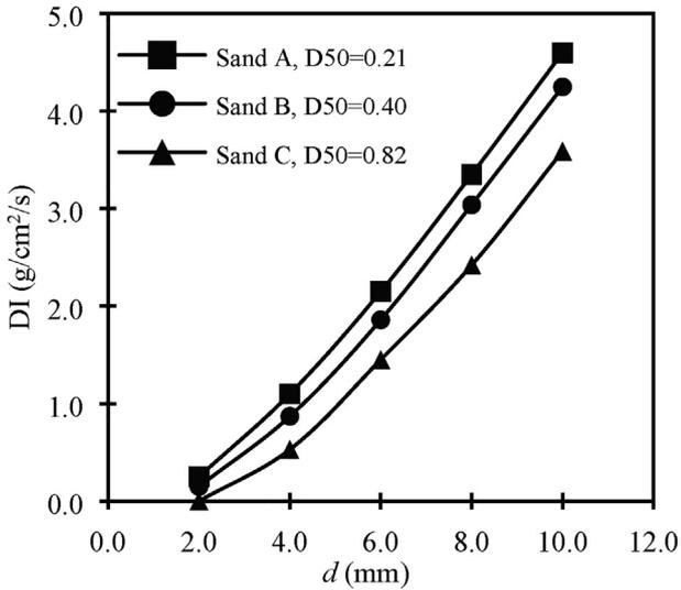
Fig. 5. Variation of DI with sieve diameter ( $d$ ) for different sand samples.
