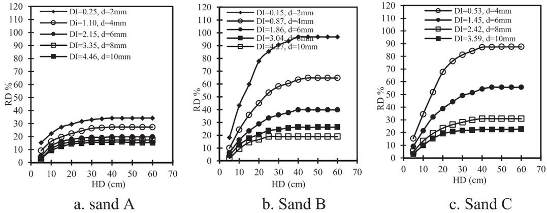
Fig. 7. Effect of the height of the drop on the relative density.
