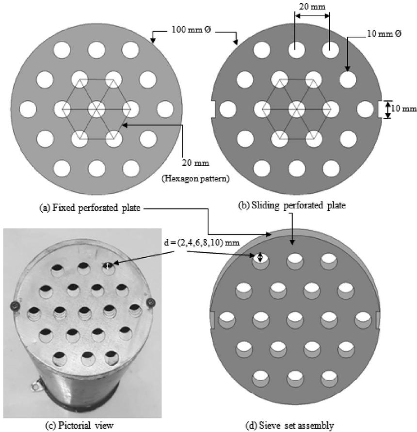
Fig. 2. Details of perforated plates used in the sieving system.
