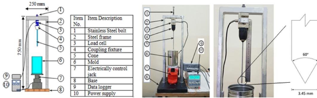
Fig. 4. Details of CPT test.
