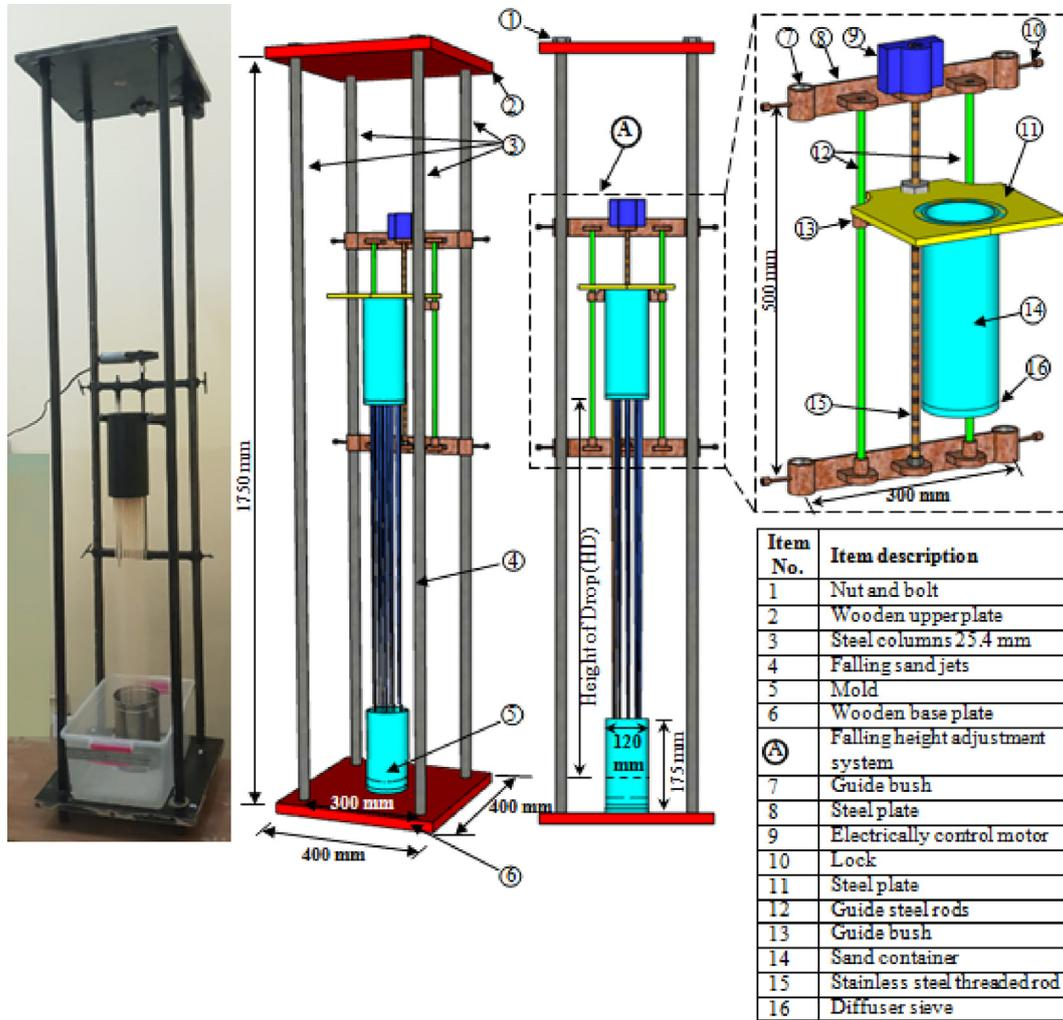
Fig. 1. Details of the Pluviation system.
