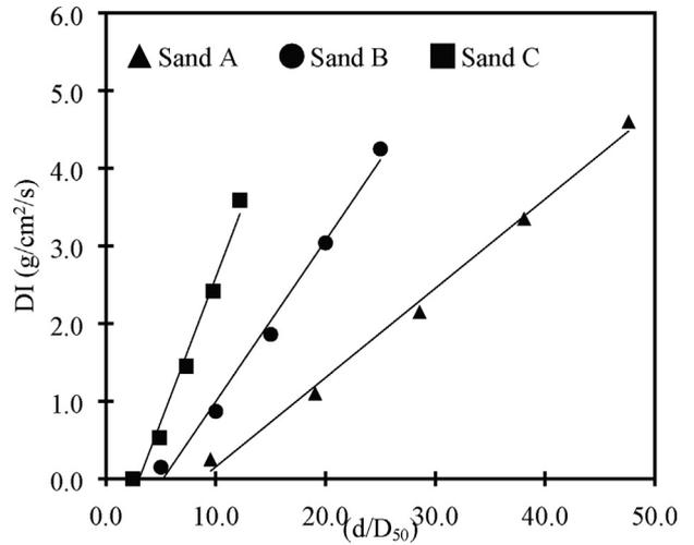
Fig. 6. Effect of  $d/D_{50}$  value on the calculated DI.
