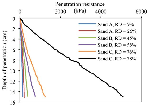
Fig. 10. CPT test results of Sand samples measured at the center.
