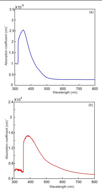
Fig. 4: Absorption coefficient of (a) ADP, and (b) MADP thin-films.
