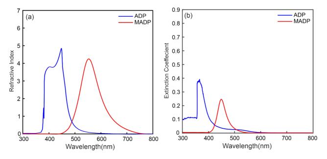
Fig. 6: (a) Refractive index and (b) the extinction coefficient of ADP and MADP samples.
