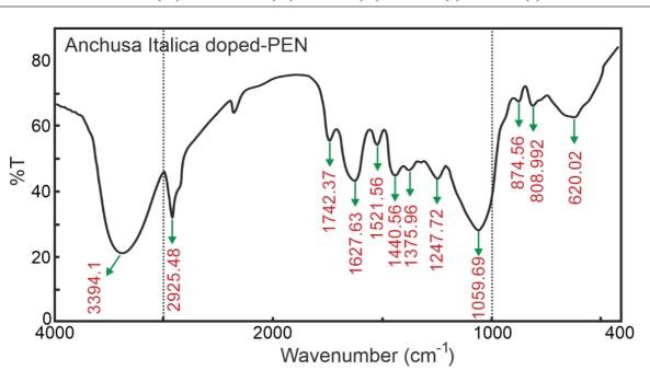
Fig. 2: Fourier transform infrared spectroscopy of dye doped polymer composites.
