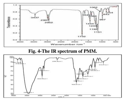
Fig. 5-The IR spectrum of the composite of PPY and PMM.
