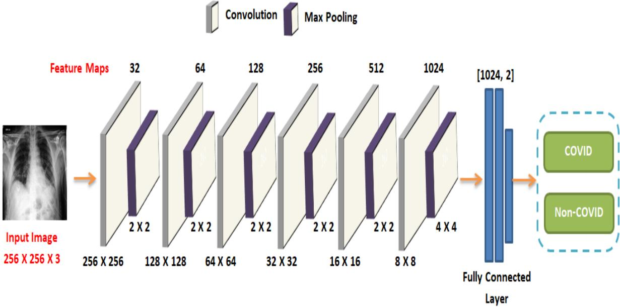
**Fig. 2. The Proposed CNN Architecture. Six Convolutional Blocks are Used.**
