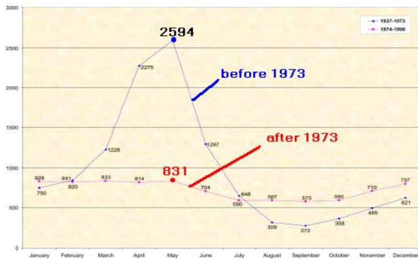
Figure (2) the discharge regime for the Euphrates river before and after 1973 periods (ACSAD, 2000 in UNEP, 2001).
