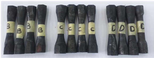
Fig. 2 illustrates the samples after quenching.
