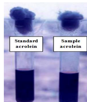
Figure 1 The color test of standard acrolein and acrolein yielded from 3-HPA dehydration.
