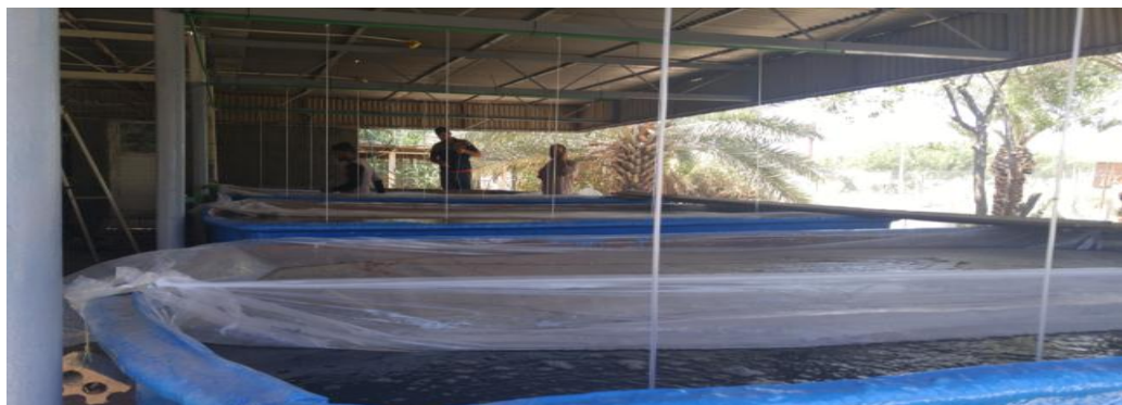
Pic. 6. Fiberglass ponds for receiving shrimp larvae and juveniles, calculating, monitoring and feeding.
