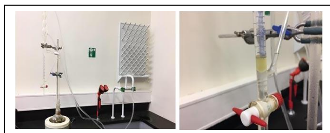
Figure 2. Clevenger apparatus for essential oil
