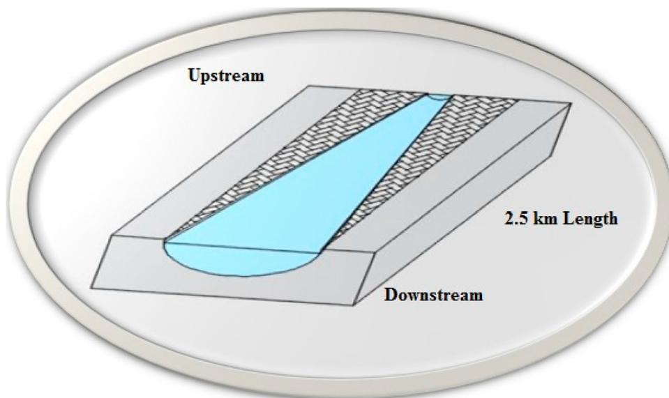
**Figure 2.** The proposed artificial concrete estuary structure.
