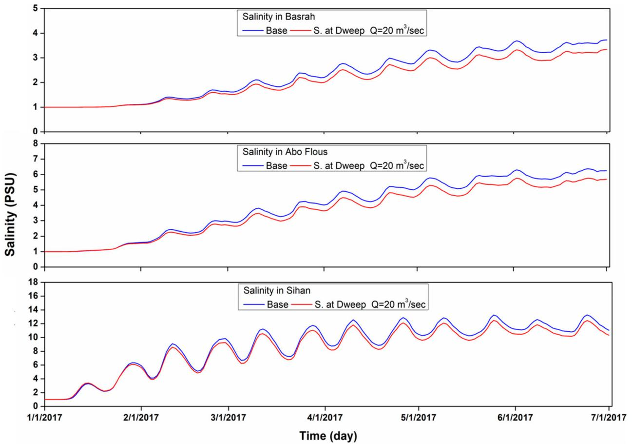
Figure 9. AD results at Basrah, Abo Flous and Sihan sites, artificial estuary at Dweeb site ( $Q = 20 \text{ m}^3/\text{sec}$ ).
