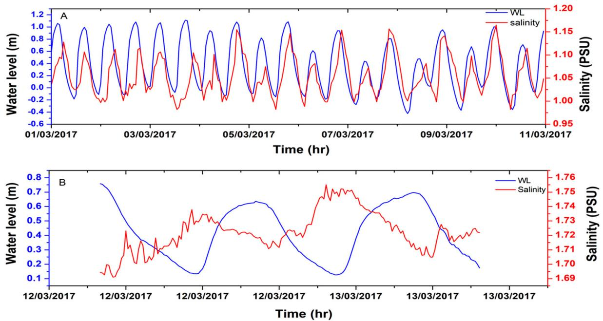
**Figure 5.** Relation of measured water level (m) and salinity of Shatt Al-Arab estuary at Sihan (A) and Abo Flous (B) sites.
