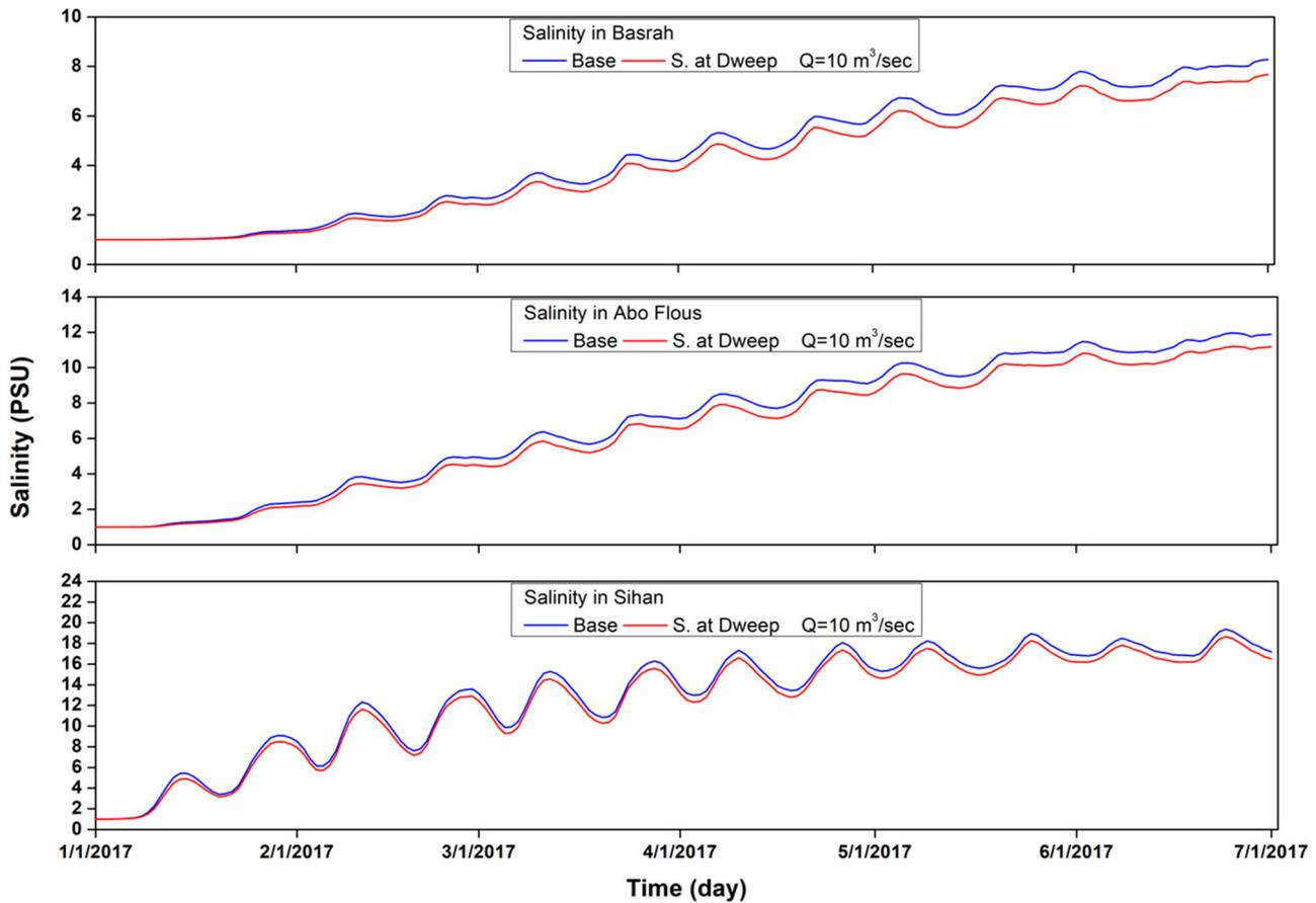
**Figure 8.** AD results at Basrah, Abo Flous and Sihan sites, artificial estuary at Dweep site ( $Q = 10 \text{ m}^3/\text{s}$ ).
