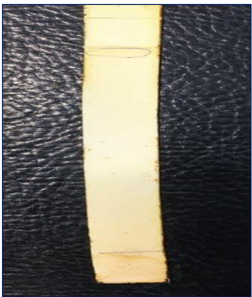
Fig. 2. Thin Layer Chromatography for terpenes component T1 with rf=0.8
