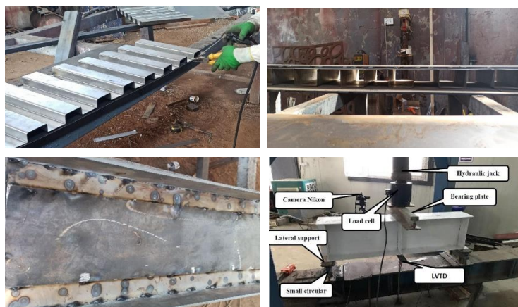
FIGURE 5. Preparation of the specimens and test setup
