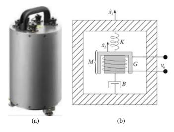
Figure 3. Broadband seismometer; (a) appearance of the device and (b) mechanical schematic
