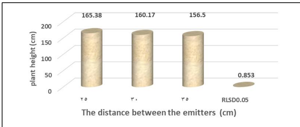
Figure (8) shows the effect of the distance between the emitters (cm) on plant height values (cm) at the end of the season.
