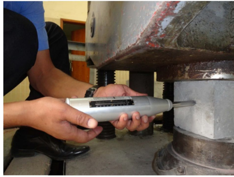
Schmidt hammer test
