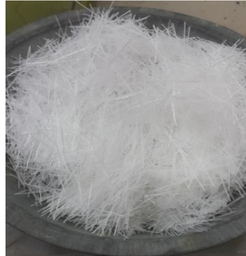
Figure 1: Polyolefin Fiber – SikaFiber® Force-60.
