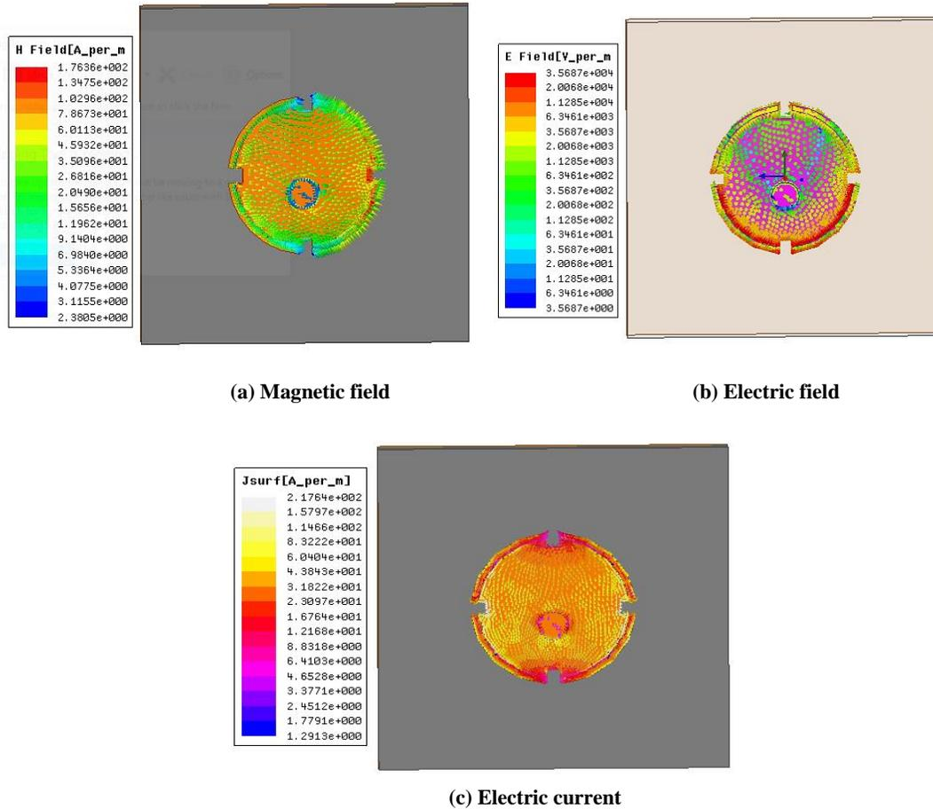
**FIGURE 9.** Magnetic and electric fields and surface distribution of electric current on the patch of the optimum suggested antenna, (a) Magnetic field, (b) Electric field , (c) Electric current.
