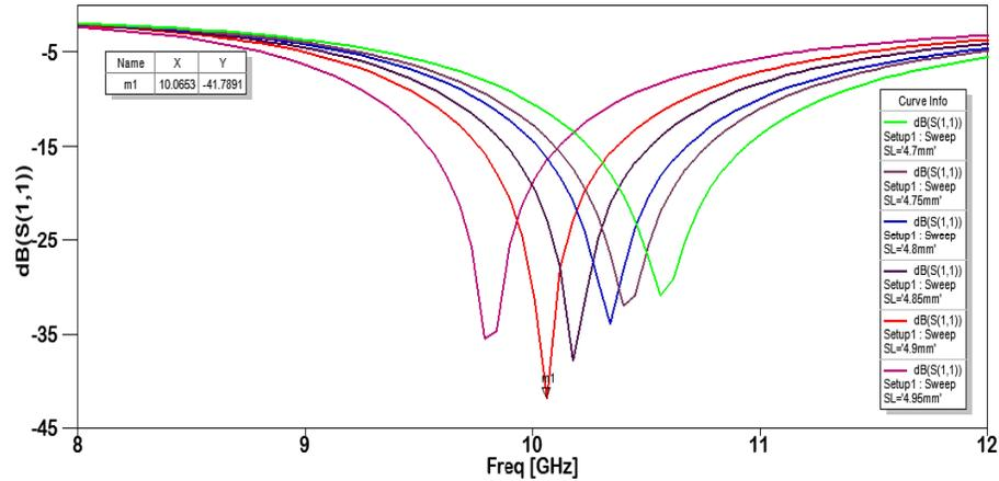
FIGURE 5. Simulation findings of the reflection coefficient for proposed design (D).
