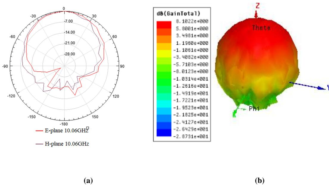
**FIGURE 8.** Simulated findings of radiation patterns of the optimum proposed design (D) at resonance frequency, (a) Two and (b) Three dimensions
