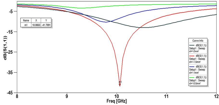
FIGURE 4. Simulation findings of the reflection coefficient for proposed design (D).
