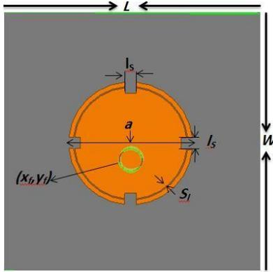
**FIGURE 2.** Geometry design of the optimum patch antenna.
