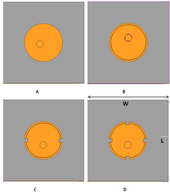
**FIGURE 1.** The steps of designed antenna. (A) CMSA, (B) annular ring slot on the circular patch, (C) two horizontal square slots on the edge of the circular patch and (D) two vertical square slots on the edge of the circular patch.
