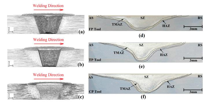
**Figure 8.** Simulation results of cross-section material flow at a joint FSWed by (**a**) FPT, (**b**) TPT, and (**c**) CPT pins. Cross-section view of a different joint area produced by (**d**) FPT, (**e**) TPT, and (**f**) CPT pins.
