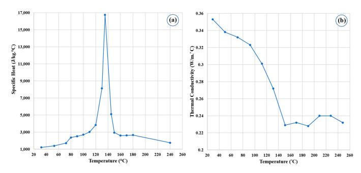
Figure 1. (a) Specific heat and (b) Thermal conductivity of HDPE.
