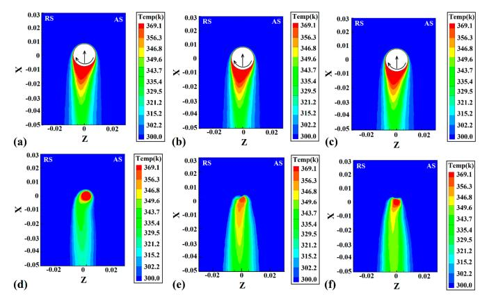
**Figure 7.** Simulation results of surface heat flow at joint FSWed by (**a**) FPT, (**b**) TPT, and (**c**) CPT pins. Simulation results of backplate heat flow at joint FSWed by (**d**) FPT, (**e**) TPT, and (**f**) CPT pins.
