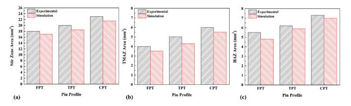
**Figure 9.** Comparison between dimensions of (**a**) stirred zone, (**b**) TMAZ, and (**c**) HAZ areas predicted by simulation and measured experimentally.
