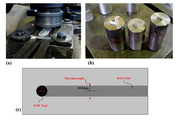
Figure 4. (a) FSW setup and joining process, (b) FSW tools, (c) Thermocouple placements.
