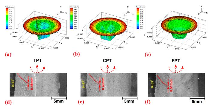
**Figure 11.** Material velocity inside the stirring zone for joints FSWed by (**a**) TPT, (**b**) CPT, and (**c**) FPT pins. Surface flow of joints FSWed by (**d**) TPT, (**e**) CPT, and (**f**) FPT pins.
