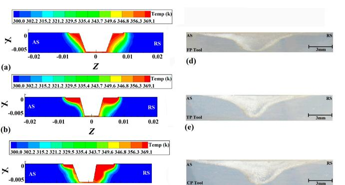
than that in the advancing side (AS). Due to the rotation of the FSW tool, the hot materials rotated from the AS to the RS, and this caused the heat concentration in the RS to be greater than in the AS. This behavior can be seen in all cases.
