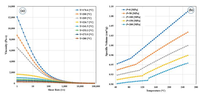
Figure 2. (a) Viscosity-shear rate and (b) Specific volume of HDPE.
