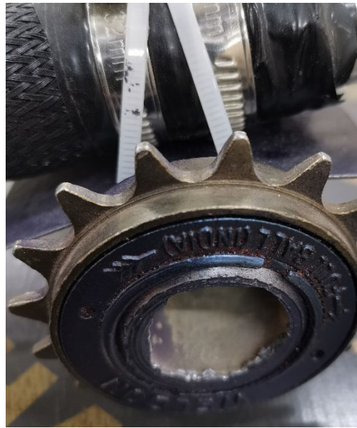
Figure 9. The freewheel to obtain unidirectional moving.
