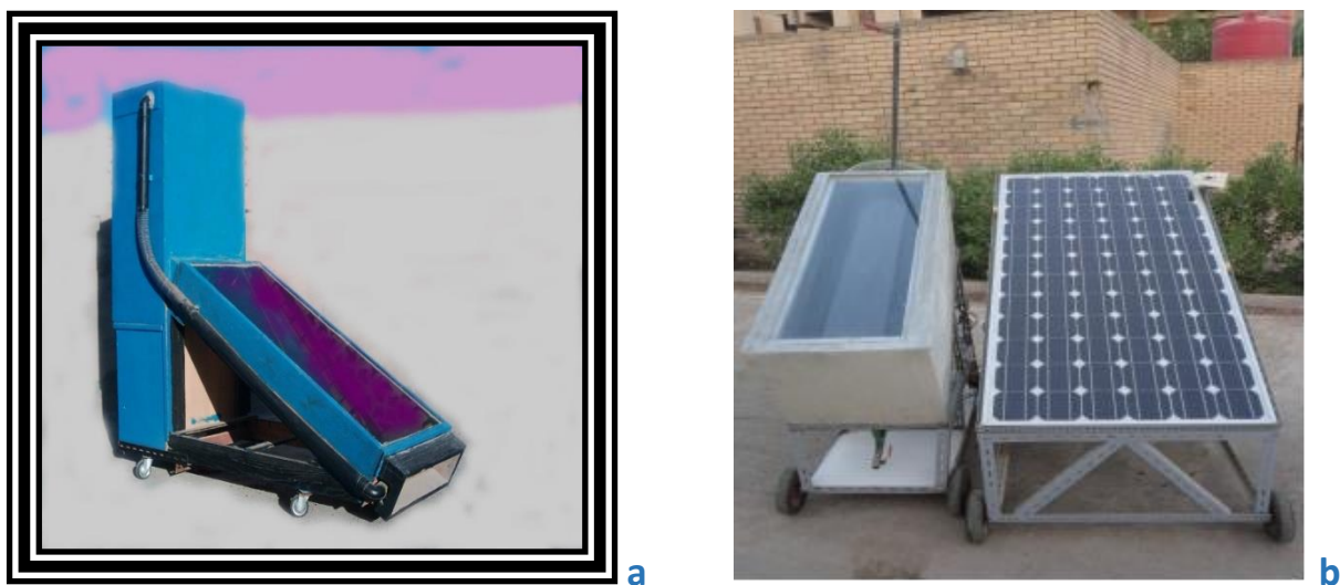
Figure 1 (a) Industrial solar dryer (Majeed and AL-Halphi 2007) and (b) Vacuum solar dryer (AL-Gwabrawy 2013).
