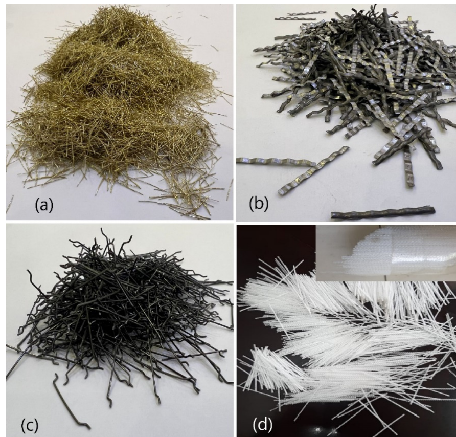
Figure 2. Types of fibers: (a) Straight steel fiber; (b) Corrugated steel fiber; (c) Hooked-end steel fiber; (d) Polyolefin fiber.
