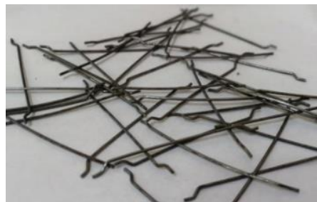
Figure 2. Steel fiber ends (Hooked)
