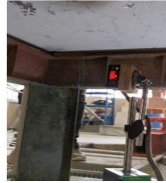
Figure 8. Deflection gage sensor
