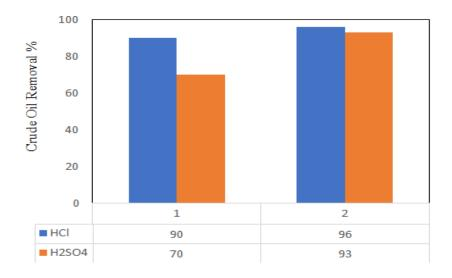
Figure 3: Effect of pH on crude oil removal percentage T=30 °C, time =1h, MCM-41 A amount (0.5g), agitation speed (400 rpm) and initial concentrations for crude oil = 50 ppm. While different pH (4, 5 and 6).
