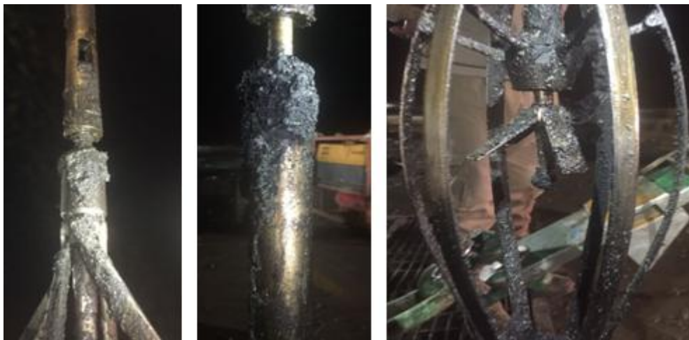
Figure 5: The Asphaltene Accumulation Effect on PLT Tool.
