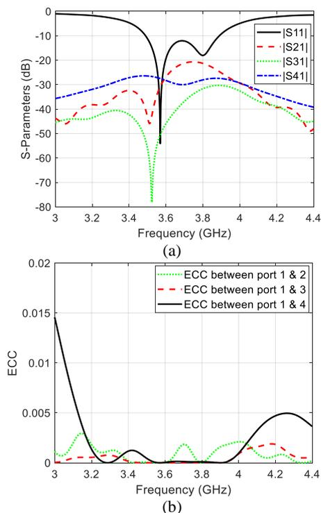
Figure 10: (a) Simulated s-parameters and (b) the ECC of the proposed MIMO antenna systems.
