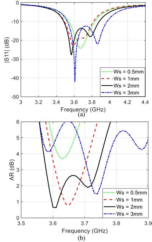
Figure 4: (a) Reflection coefficient and (b) broadside AR of the antenna with chip resistors at  $dr = 1.5mm$  and different values of  $W_s$ .
