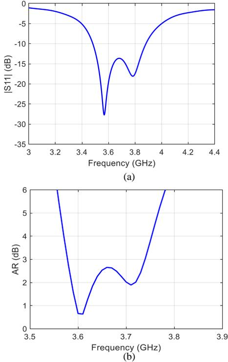
Figure 6: Simulated (a) Reflection coefficient and (b) broadside AR of the antenna with chip resistors.
