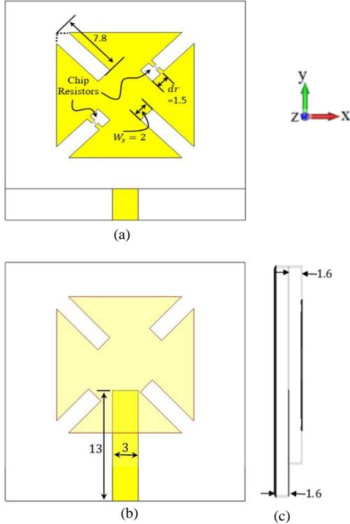
Figure 1: The structure of the broadband CP antenna with chip resistors with its optimized parameter values (a) top view, (b) the feed line structure, and (c) the side view. (All dimensions are in mm).
