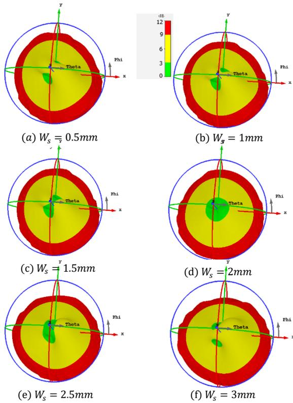
Figure 3. The axial ratio pattern of the antenna with chip resistors for various values of slit width at 3.6 GHz.
