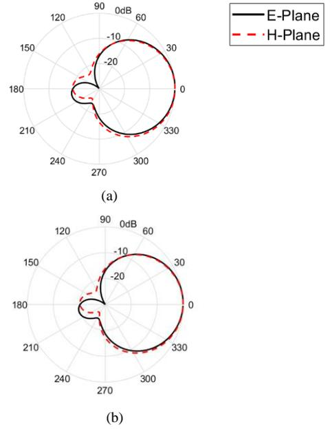
Figure 8: The power pattern of the antenna with chip resistors at (a) 3.6GHz and (b) 3.7GHz.
