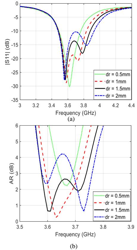
Figure 2: (a) Reflection coefficient and (b) broadside AR of the antenna with chip resistors at different values of  $dr$ .
