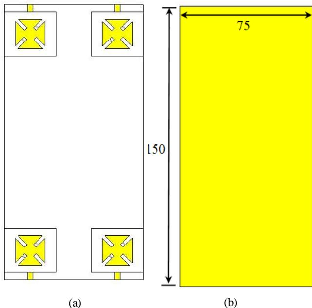
Figure 9: The proposed MIMO structure (a) top view and (b) the back view. (All dimensions are in mm).
