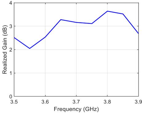
Figure 7: Simulated realized gain of the antenna with chip resistors as a function of frequency.
