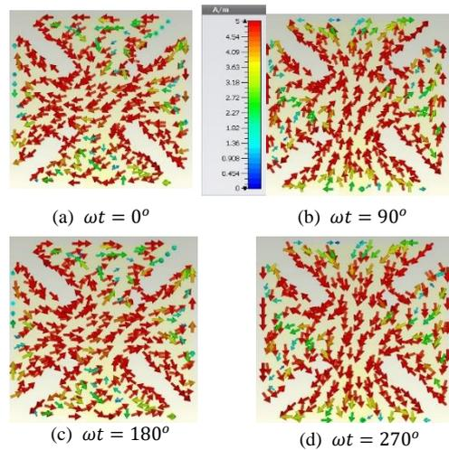
Figure 5: The current distribution on the radiating patch of the antenna with chip resistors for different time instants at  $f = 3.6GHz$ .
