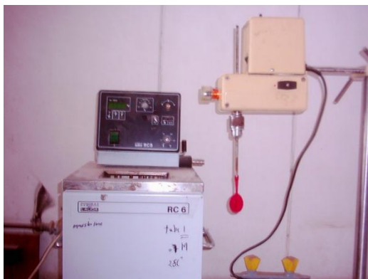
Figure 2: Electric mixer with four blades, plastic impeller
