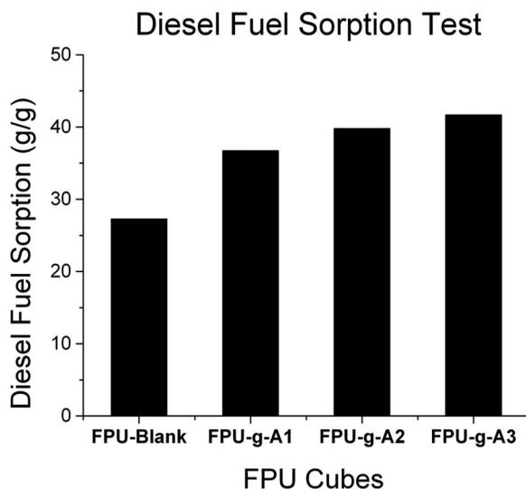
**Figure 3.** The sorption capacity of diesel fuel of the blank FPU cubes and modified FPU cubes.**Table 3.** The water sorption capacity of the blank FPU cubes and modified FPU.
