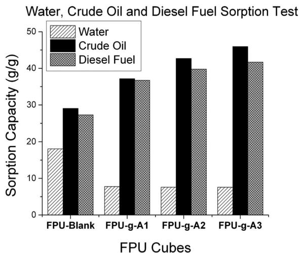
**Figure 5.** Water, crude oil, and diesel fuel sorption capacities of the blank FPU cube and modified FPU cubes.
