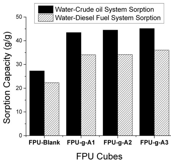
**Figure 8.** Crude oil and diesel fuel sorption capacity of the blank FPU cube and modified FPU cubes.
