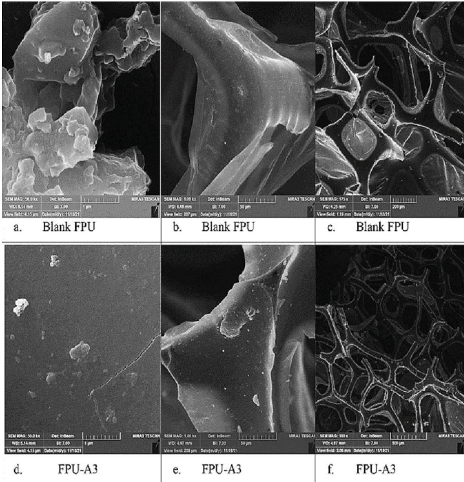
**Figure 1.** SEM micrographs of the blank FPU cubes (a–c) and modified FPU cubes (d–f).
