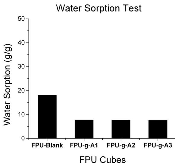
**Figure 4.** The water sorption capacity of the blank FPU cubes and modified FPU cubes.
