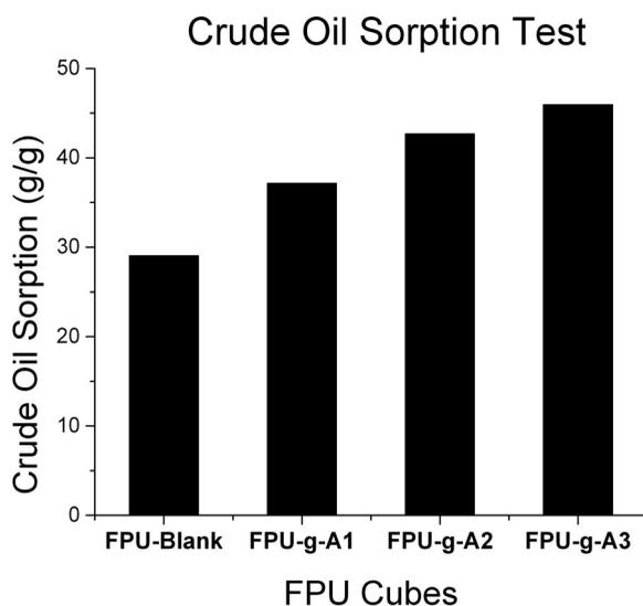
**Figure 2.** The crude oil sorption capacity of the blank FPU cubes and modified FPU cubes.
