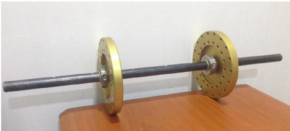
Figure 8. Rotor assembly: shaft, disks, two-piece shaft collars.
