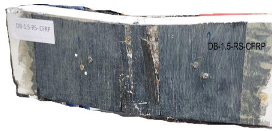
Figure (12): Failure mode for Rehabilitated Deep Beam with (a/d=1.5) failed in shear - DB-1.5-RS-CFRP
