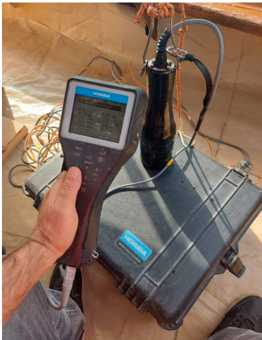
Figure 2. Measuring the salts concentration in the field using a Horiba U-10 device.
