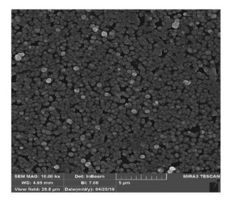
Figure 3. FESEM images of CdSe NPs.
