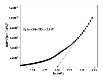
Figure 6. Band gap of CdSe thin films deposited on glass.
