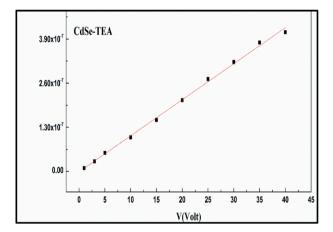
Figure 9. Plot showing variation of current voltage.
