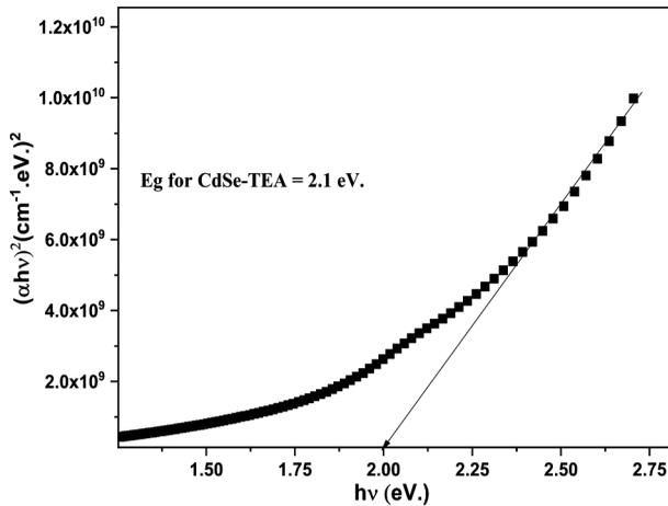
**Figure 6.** Band gap of CdSe thin films deposited on glass.
