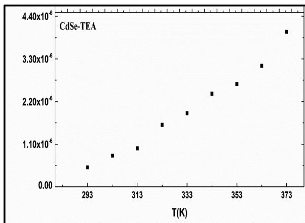
**Figure 10.** Variation of conductivity with temperature.
