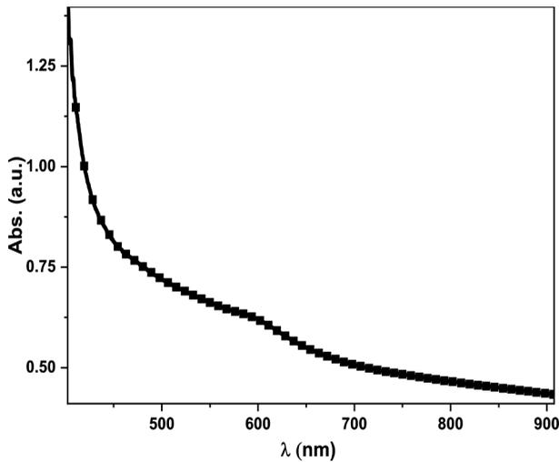
Figure 5. Absorption spectrum of CdSe thin films deposited on glass.
