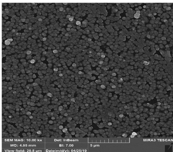
**Figure 3.** FESEM images of CdSe NPs.
