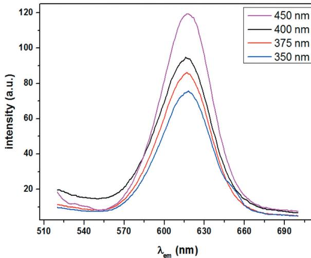
**Figure 7.** Photoluminescence spectra of CdSe-TEA nanoparticles at different excitation wavelength.
