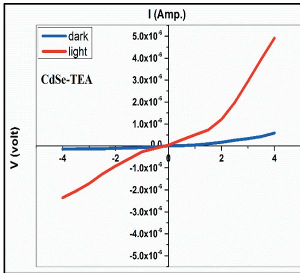
**Figure 12.** I–V characteristics of an AL/CdSe-TEA/Ag photodetector in darkness and illumination.
