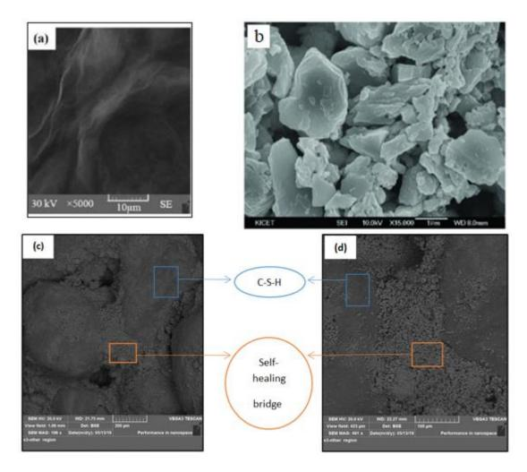
Fig. 9. (a) SEM of base mortar, (b) SEM of cement powder, (c) & (d) SEM for bio-mortar with (5ml) Nutrient broth Proteus.
