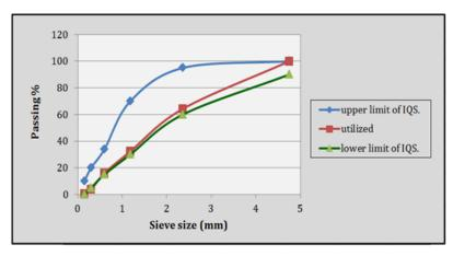
Fig.1. Grading of natural sand Iraqi Specifications Measurement...(1984/45).
