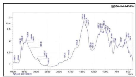
Fig.7. FTIR test for bio-mortar with (25ml) of Nutrient broth Proteus bacteria.
