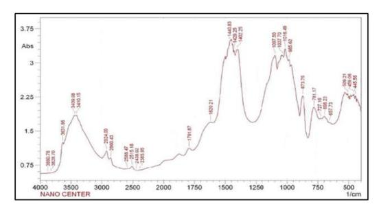
Fig. 5. FTIR spectrum of cement mortar with 5ml of BHI E.Coli bacteria
