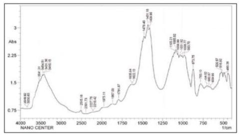
Fig. 6. FTIR test for bio-mortar with (25 ml) of Nutrient broth E.coli bacteria.
