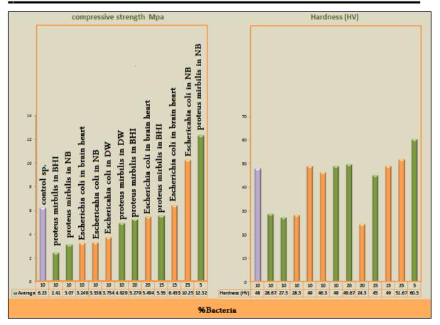
Fig. 3. Compressive strength for bio-(N-type) mortar. Fig. 4. Hardness test for bio-(N-type) mortar.
