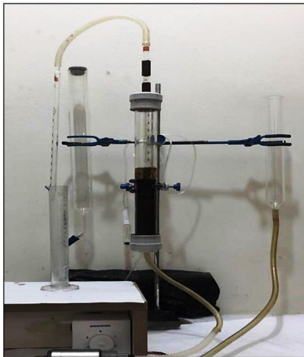
Figure 2: sand-pack column used for MEOR studies adapted of (Suthar et al. , 2008).
